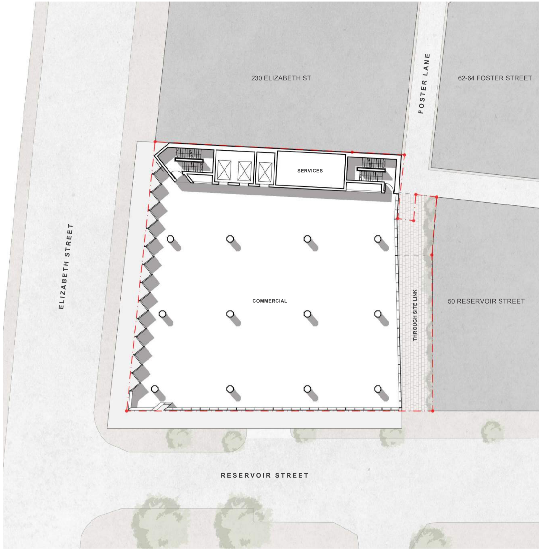
TYPICAL FLOOR PLAN - L1 TO L7 COMMERCIAL GFA 714 m 2
